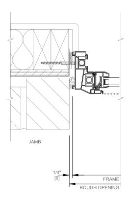
SEE INSTALLATION INSTRUCTIONS FOR ANCHORAGE SCREW SIZE, LOCATION AND SPACING
