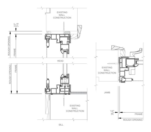
FLASHING BY OTHERS Metal head flashing. Metal sill flashing.
