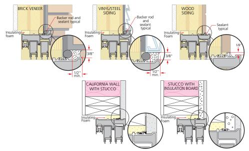
Note: Application of closed cell foam backer rod and sealant does not apply to stucco.
