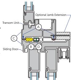
E. Apply sealant to the ends of the mullion joint. The bead of sealant should extend from the center of the mullion joint to the exterior of the unit, covering the foam plug.
