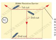
Make a 6" cut up from each top corner at a 45° angle to allow the water resistive barrier to be lapped over the fin at the head of the door.
