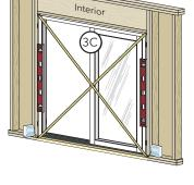
E. Install roller retainers. Position and secure the two roller retainers provided by drilling pilot holes through the pre-drilled holes into the sill support. Apply sealant to the holes and insert screws as specified below:
