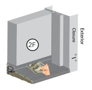
G. If needed the height of the standard threshold can be adjusted to achieve appropriate contact with the door sweep. Remove the screw cover caps as necessary and use a #2 Phillips screwdriver to turn the adjustment screws clockwise to lower the threshold or counterclockwise to raise the threshold.
