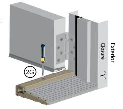
H. Remove the backing paper from the corner seal pads and place one in each corner of the frame tight against the top of the threshold and thicker portion of the tapered pad against the frame weatherstrip.
