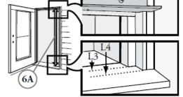
**Starting** at the top of the latch mounting frame, mark off your measurement (see 6A) and cut to length matching the angle of the sill.
