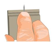
D. Using the tack insertion tool, locate the tack in-line with the pencil mark. Push the tack into the wood until it is stops.
