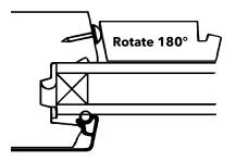
F. Install the grille into the window, bottom first.
