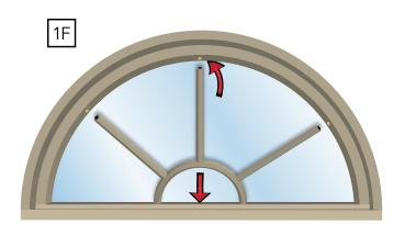
G. Secure grille bars by applying direct pressure to each end bar over the tack.
