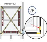
**Double-Hung:** Cut the checkrail bands (if applicable) and remove shipping spacers. Open, close and tilt the sashes to test for proper operation. Check for equal sash to frame reveal from top to bottom.
