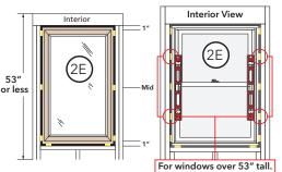
NOTE: DO NOT shim above the window or between the sill shims. Additional shims are required at screw locations for large units and combinations. See the anchor instructions at the end of this booklet.
