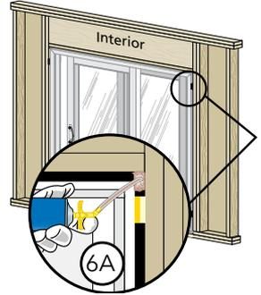
**Note:** It may be necessary to squeeze the end of the tube with pliers to be able to insert into the space between the door frame and the rough opening. DO NOT completely fill the space from the back of the fin to the interior face of the door.
