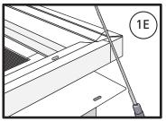
F. Using a utility knife, score (3 times) the point where the J-mould attaches to the exterior face of the product. Beginning at one end of the J-mould, grasp the J-mould with pliers and bend the J-mould toward the interior of the product. Continue along the entire length of the product until the J-mould is removed from the product.
