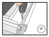
G. Using a utility knife, cut off any excess material that does not break off the accessory groove.
