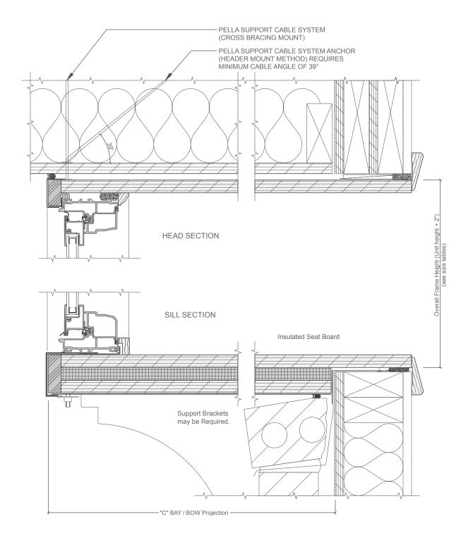
(1) The Bay/Bow support cables must be attached to structural members capable of supporting 1,300 lbs. Knee braces are required in addition to the support cables if the structural members are not capable of supporting 1,300 lbs. Bay/Bow units are not designed to support roof structure.
