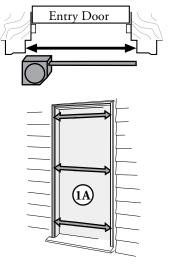
B. **If required, shim the entry door frame.** Using four shim sections each about 8" to 12" long, position to align with the hinges on the storm door. DO NOT extend the shim beyond the face of the entryway. (Shims not provided)
