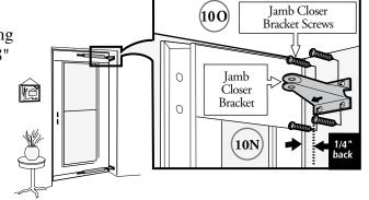
Note: Removing the door jamb bracket from the closer may make installation of the bracket easier.
