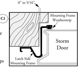
Hint: Drilling and installing the top screw first makes it easier to align the mounting frame correctly.
