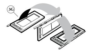
H. Matching the angle of your entryway sill, cut the bottom of the hinge mounting frame to length.
