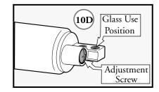
D. Attach the door closer to the door closer bracket using the long closer pin in the "glass use" position and turn the adjustment screw counter clockwise 4 to 5 turns.
