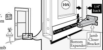
B. **Install the bottom jamb closer brackets** using four jamb bracket screws (#10 x 1-1/2" Phillips pan head) for each bracket.
