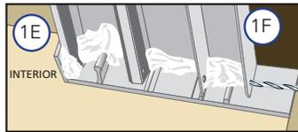
F. Place a bead of sealant at each joint where the existing door frame jambs meet the existing door sill pieces. Fill any holes in the jamb and head with sealant.
