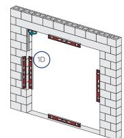
E. **Measure and mark the opening** where the interior of the new door will be placed. Consider the size of wall cavity (if applicable) and 3/4" minimum overlap onto the brick veneer or finished wall materials for exterior perimeter sealant.
