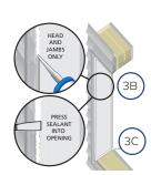
C. Place a 3/8" bead of sealant at each corner of the opening.
