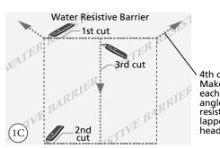
4th cut: Make a 6" cut up from each top corner at a 45° angle to allow the water resistive barrier to be lapped over the fin at the head of the door.
