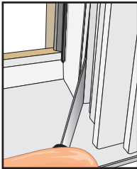
Pry off Monumental Double-Hung jamb liner
