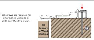
Remove screw cover. Drive screws at each pre-punched hole or drill pilot holes if none are present. Add sealant in each pre-drilled hole before driving screws. Reinstall screw cover.
