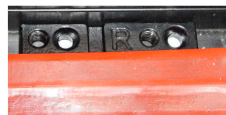
RH Bottom plate installed in sill track
