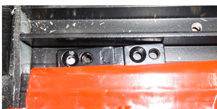
LH Bottom plate installed in sill track
