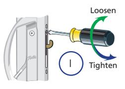
I. **Install the keeper** by inserting 3" long screws (provided) through the keeper holes, the shim and into the rough opening frame members. Remove the starter screw from the 4 screw hole keeper and replace it with a 3" long screw.
