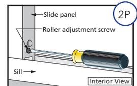
**NOTE: For doors with heavy impact-resistant or triple pane glass use a small pry bar to raise the panel while turning the adjustment screw. This will prevent the threads from being stripped.**
