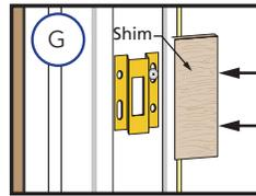
H. **Adjust the lock hook** by turning the door lock adjustment screw clockwise to loosen or counter-clockwise to tighten until the mortise lock is aligned properly, the door locks easily, and there is less than 1/16" movement when the door is locked.
