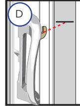
F. **Place the keeper with 2 screw holes** on the jamb by "snapping" it into the frame jamb at the desired location. The keeper may be moved up or down to align with the pencil mark. The keeper will stay in position until attached with screws.
