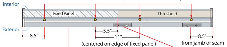
Exterior sill edge must be supported to meet performance values. Apply Pella aluminum sill support or wood blocking as required to support the exterior edge of the door frame.
