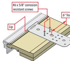
Alternatively, it is acceptable to use two #6 x 5/8" screws through the clip with the clip on its back and not engaged in the fin groove.
