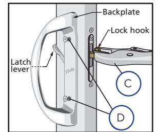
E. **Remove the mortise lock.** Remove the two screws that attach the lock assembly to the door panel. Work the lock down, then tilt it out and pull up.
