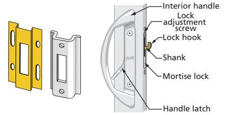
E. **Place the keeper with 4 screw holes** on the jamb so the top of the slot is aligned with the pencil mark. Attach by inserting a #6 x 1/2" starter screw into one of the slotted keeper holes.
