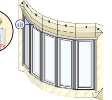
C. **Fold down the top flap** of the water resistive barrier.
