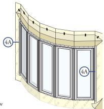
B. **Apply top flashing tape.** Cut a piece of flashing tape long enough to go across the top of the window and extend at least 1" past the side flashing tape on both sides. Apply the tape over the top nailing fin as shown. Press the tape down firmly.
