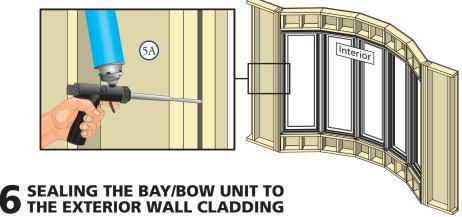
When applying siding, brick veneer or other exterior finish material, leave adequate space between the window frame and the material for sealant.
