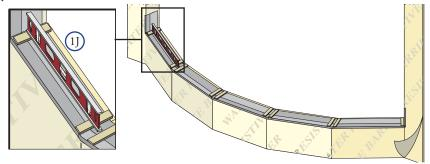
K. Remove plastic wrap, plywood, blocking and handles from window. DO NOT unlock or open the windows until it is shimmed square and plumb in the opening.
