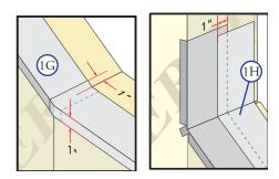
H. **Apply sill flashing tapes #2.** Starting with the flashing tape for one sill end, cut a piece 8" longer than the end unit width.
