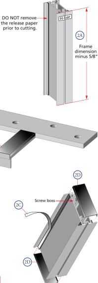
E. Fasten the prepared mullion cap to the H-bar using four #8 x 1" flat head screws. Be sure to drive the screws into the H-bar screw bosses as shown. This can be assured by aligning the back of the cap to the outer surface of the H-bar. Repeat this step for the other end.
