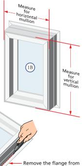
Remove the flange from the unit on the side that will receive the mullion.
