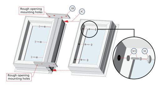
F. Apply high quality exterior grade polyurethane or silicone sealant to both ends of the mull as shown.
