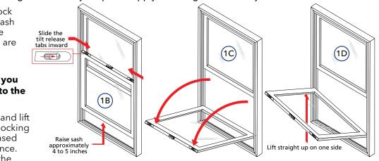
locking pivot bar is released from the opposite side of the sash and can be removed from the bottom of the balance. Lift the sash up and out of the window frame. Set it aside in a safe location.
